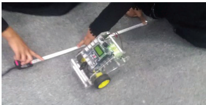
Figure 2: Robotics, STEM and computational thinking: students explore a robot’s velocity by measuring the distance X (Cm) the robot moves on the floor over Time (sec).
